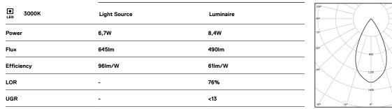
Beam angle Flood 52° Application Units 39° Weight 0,3Kg
