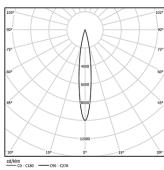
Beam angle Spot 15° Application Weight 0,58Kg
