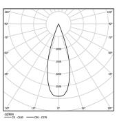
Beam angle Medium 41° Application Weight 0,64Kg
