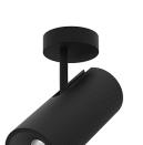
Design: O/M + Bartenbach GmbH Surface spotlight with die-cast aluminium body with electrostatic 100% polyester paint finish. Spot-lens with individual complex surface rips to provide a focal light and an extremely narrow beam. Orientable by 90° horizontal rotation and 330° vertical rotation.
