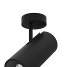
Design: O/M + Bartenbach GmbH Surface spotlight with die-cast aluminium body with electrostatic 100% polyester paint finish. Spot-lens with individual complex surface rips to provide a focal light and an extremely narrow beam. Orientable by 90° horizontal rotation and 330° vertical rotation.
