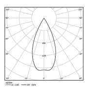
Beam angle Flood 59° Application Weight 0,64Kg
