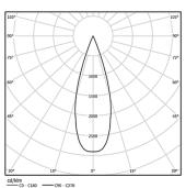
Beam angle Medium 41° Application Weight 0,64Kg
