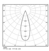
Beam angle Medium 41° Application Weight 0,64Kg
