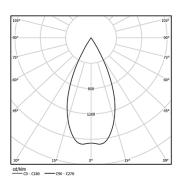
Beam angle Flood 59° Application Weight 0,64Kg
