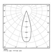
Beam angle Medium 41° Application Weight 0,64Kg
