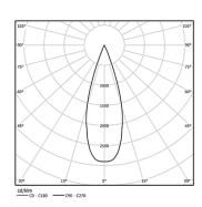
Beam angle Medium 41° Application Weight 0,64Kg
