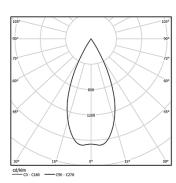
Beam angle Flood 59° Application Weight 0,64Kg
