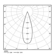
Beam angle Medium 41° Application Weight 0,64Kg
