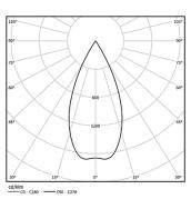
Beam angle Flood 59° Application Weight 0,64Kg
