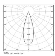
Beam angle Medium 41° Application Weight 0,64Kg
