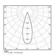
Beam angle Medium 41° Application Weight 0,64Kg
