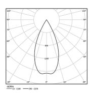
Beam angle Flood 59° Application Weight 0,64Kg
