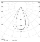
Beam angle Flood 64° Application Weight
