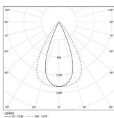
Beam angle Flood 64° Application Weight
