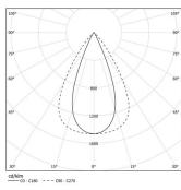
Beam angle Flood 64° Application Weight
