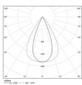
Beam angle Flood 64° Application Weight
