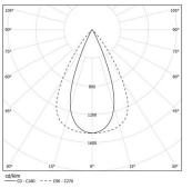
Beam angle Flood 64° Application Weight 4,7Kg
