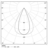
Beam angle Flood 64° Application Weight
