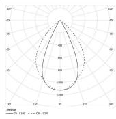
Beam angle Wide flood 76° Application Weight
