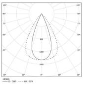
Beam angle Flood 64° Application Weight
