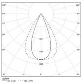
Beam angle Flood 64° Application Weight 4,7Kg
