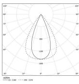
Beam angle Flood 64° Application Weight
