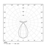
Beam angle Flood 64° / batwing
