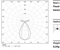
Beam angle Flood 64° / batwing
