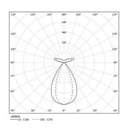
Beam angle Flood 64° / batwing
