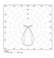
Beam angle Flood 64° / batwing
