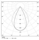
Beam angle Wide flood 76° Application Weight
