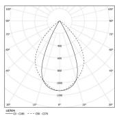
Beam angle Wide flood 76° Application Weight
