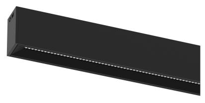
Design: OM + Bartenbach GmbH Surface or pendant luminaire with housing made of aluminium with 25 micron maximum corrosion resistance anodization in matte finish or electrostatic 100% polyester paint with textured finish. Aluminium anodised end caps with matt finish or electrostatic 100% polyester paint with textured-
