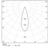
Beam angle Medium 31° Application Weight 2,4Kg
