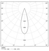
Beam angle Medium 31° Application Weight 2,4Kg
