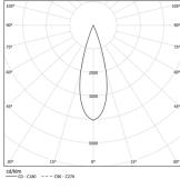
Beam angle Medium 31° Application Weight 2,4Kg
