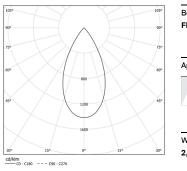
Beam angle Flood 52° Application Weight 2,4Kg
