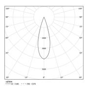
Beam angle Medium 30° Application Weight 0,8Kg
