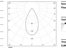
Beam angle Flood 52° Application Weight 0,8Kg
