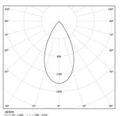
Beam angle Flood 50° Application Weight 0,5Kg
