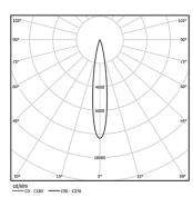
Beam angle Spot 12° Application Weight 0,6Kg
