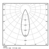
Beam angle Medium 28° Application Weight 0,6Kg
