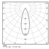
Beam angle Medium 28° Application Weight 0,6Kg
