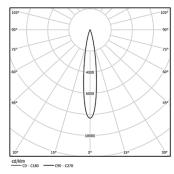
Beam angle Spot 12° Application Weight 0,6Kg
