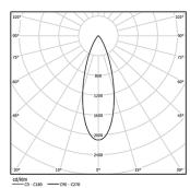
Beam angle Medium 28° Application Weight 0,6Kg
