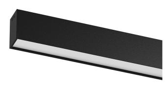
Design: Eduardo Souto de Moura Surface or pendant luminaire with housing made of aluminium profile with 25micron maximum corrosion resistance anodization with matt finish or with textured electrostatic 100% polyester paint. Frosted polycarbonate diffuser with user friendly clipping system and double fitting system: flushed or recessed.
