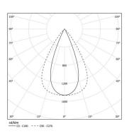
Beam angle Flood 65° Application Weight
