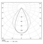
Beam angle Wide flood 80° Application Weight
