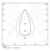
Beam angle Flood 65° Application Weight
