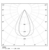
Beam angle Flood 65° Application Weight
