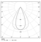
Beam angle Flood 65° Application Weight
