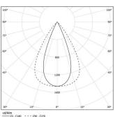
Beam angle Flood 65° Application Weight
