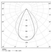
Beam angle Wide flood 80° Application Weight
