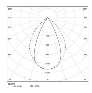
Beam angle Wide flood 80° Application Weight
